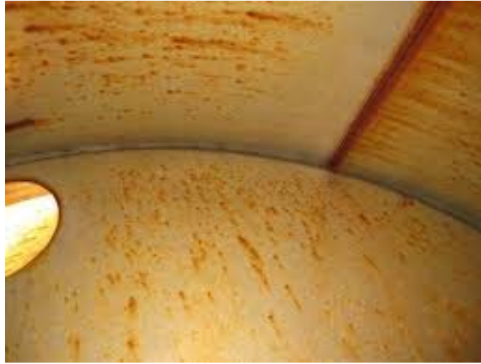
Stainless Steel Tank non Passivated
