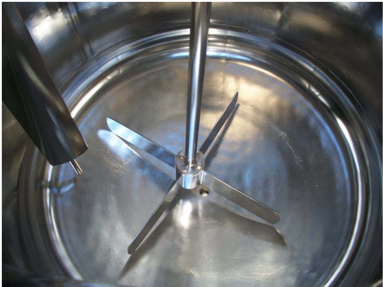
A well passivated stainless steel tank
